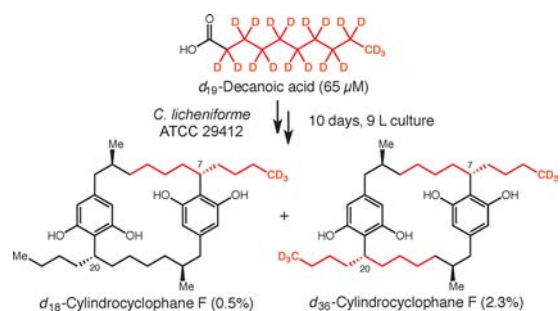
Figure 5. Incorporation of labeled decanoic acid into cylindrocyclophane F by C. licheniforme .
